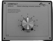
Caution: the HP-COMPACT will not limit if an appliance draws more current than available from the source! This means that the connected generator will be overloaded or that the circuit-breaker before the HP-COMPACT will break.
